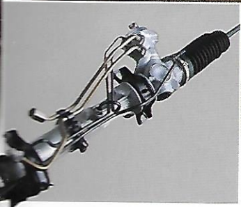
Power Rack-and-Pinion Steering Escort's precise rack-and-pinion steering system is power assisted with a 17:1 steering ratio for ease of maneuverability.
