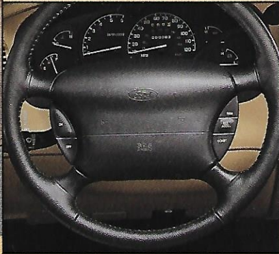
Ranger speed control has a feature that lets you increase your speed in increments of one mile per hour.
