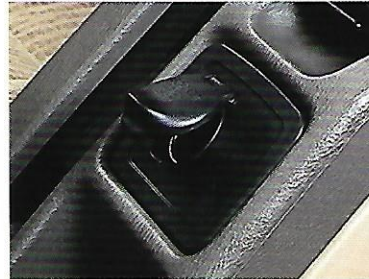
Power outlet. Auxiliary 12v outlet for additional power. Excludes All Weather Package and 5MT.
