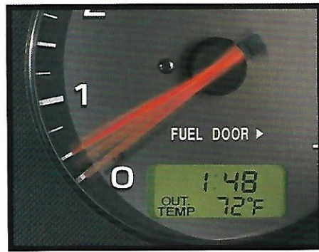
An ambient temperature gauge is located below the clock on the instrument panel to keep the driver aware of the outside temperature.
