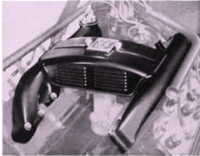
The carburetor heat deflector is a smart finishing touch on the engine
