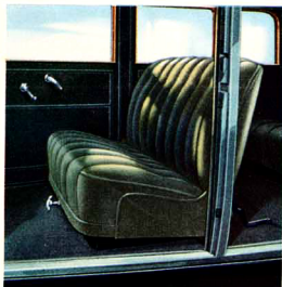
Front seats in all closed models are fully adjustable forward and back by an easy turn of the conveniently located control
