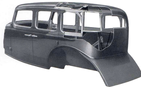
Steel welded into a single mighty unit and reinforced with resilient hardwood makes the Fisher body of the Oldsmobile strong, durable, safe. This cutaway picture shows how the steel body is reinforced at every point where extra strain occurs.
