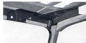
This heavy bracing between the front pillar and the top cross bar of the body frame is typical of the extra strength in all parts of Oldsmobile's Fisher bodies.
