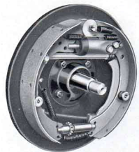
The internal construction of the brakes is identical with that of the highly efficient, self-energizing brakes used by Oldsmobile during the past three years, except that the brake is now actuated by a piston in an hydraulic cylinder.
