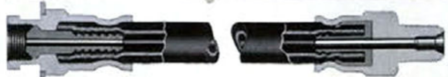
HOSE AND TUBING CONSTRUCTION —Note the extreme simplicity and trouble-proof construction of Chevrolet's Perfected Hydraulic Brakes. Three identical, flexible hoses are used to connect the hydraulic piping to the front wheel cylinders and the lines leading to the rear cylinders. Each consists of strong, durable hose, with leak-proof joints, capable of withstanding pressure up to 2500 pounds.
