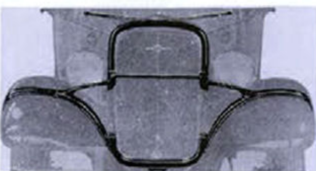
STABILIZED FRONT END —Mounted as a unit, the front fenders, radiator and headlamps are free of counter-strain and excessive movement. This construction not only protects the radiator core and prevents squeaks and rattles, but stabilizes the front-end balance and gives easier, safer driving on rough roads.
