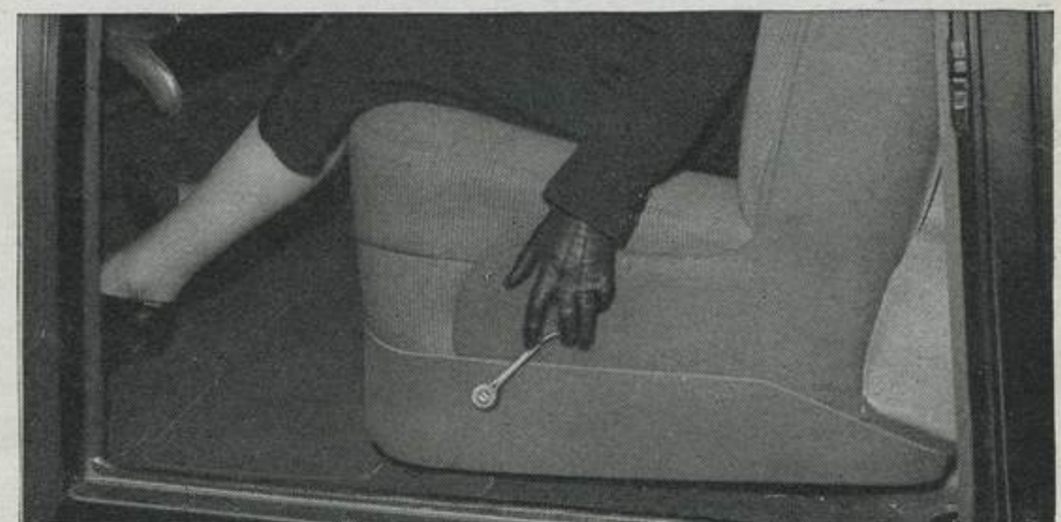
Just trip this convenient release and you can adjust the front seat to a perfect fit, without taking your eyes off the road. The seats rise and tilt slightly as they are moved forward, offering perfect accommodations for the smallest driver
