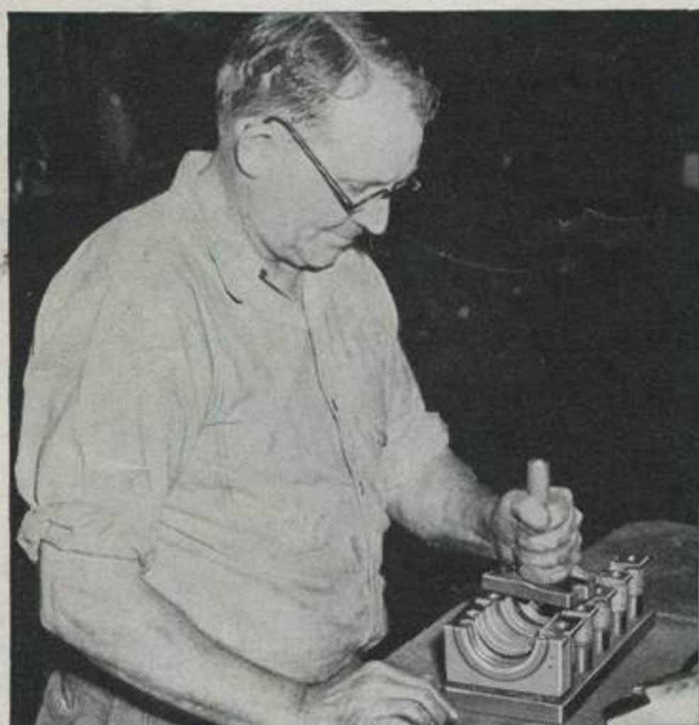
Colin McLeod has been with Buick for thirty-one of his fifty-seven years. He puts finishing touches on the main bearings
