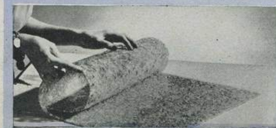
It took over six years of research and six million dollars to develop the new safety plate glass that Buick uses. See how this eye-saving new glass (A) compares with ordinary safety sheet glass (B) in the unretouched photographs at right. Notice, too, that no matter how much it's hammered the new safety plate glass can be rolled up like a carpet, as shown at left—the improved inner layer of plastic still holds all the glass fragments
