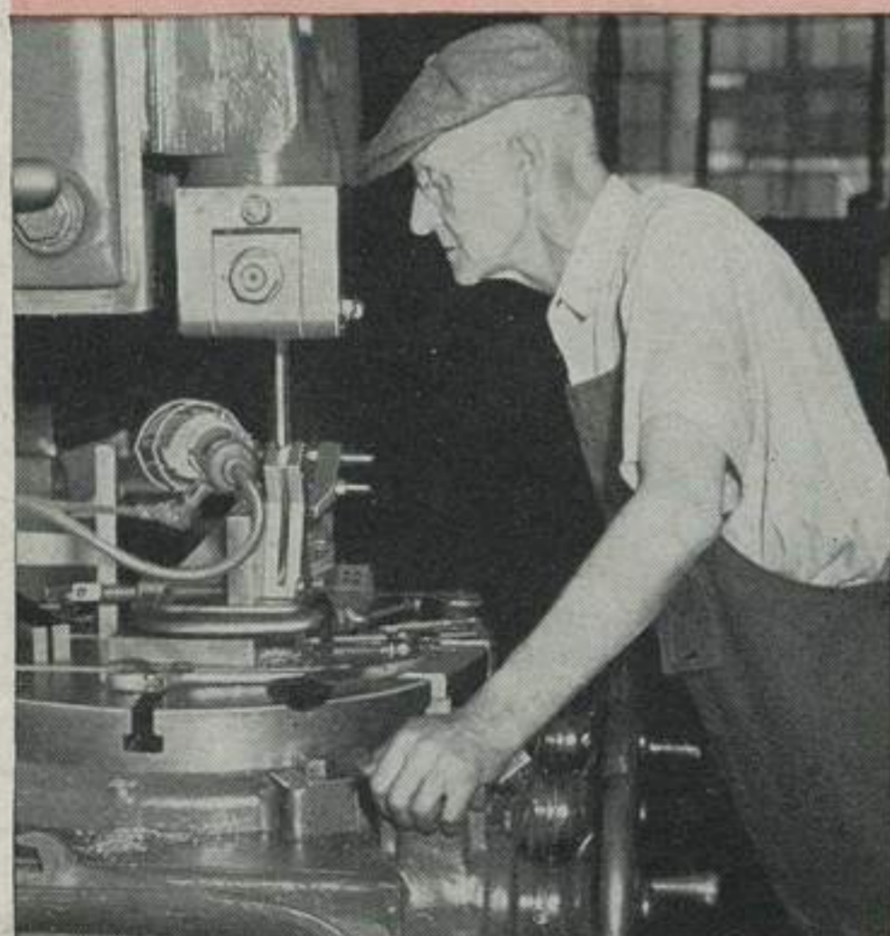
Claude C. Baldwin, with nineteen years of Buick service to his credit, is a skilled tool-maker. He is shown at a slotter machine
