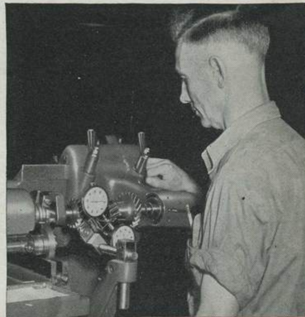
Harry Pearson, Buick man for fifteen years, checks the lead on a counter gear, using one of Buick's modern precision machines
