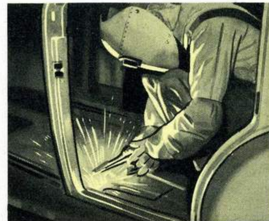
"Welding fuses the roof, floor, sides, front and back of the steel bodies into a solid whole."
