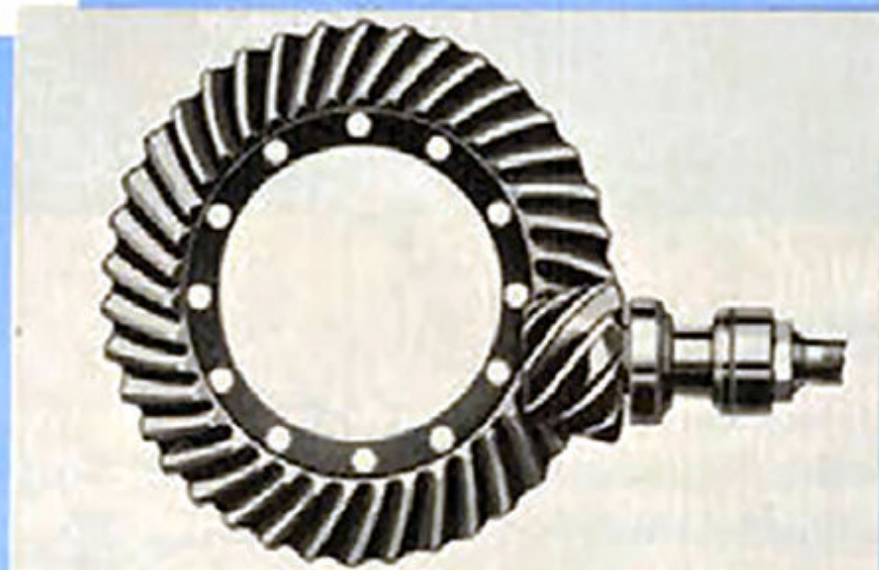
Rear Axle —Hypoid drive gears give a new maximum of strength and durability. Differential bearings are barrel roller type.
