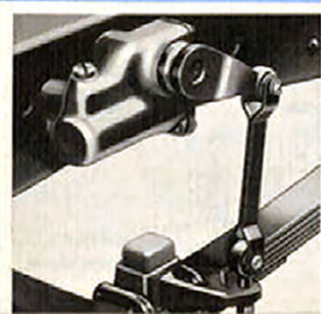
Shock Absorbers —Delco hydraulics, single-acting front and rear, add to driver comfort, protect the truck and its load, and give more positive steering control.
