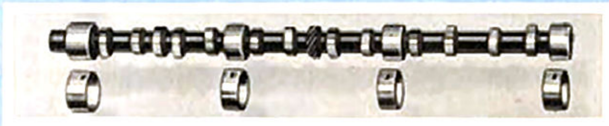
Camshaft —The four-bearing camshaft of drop-forged steel runs on four steel-backed babbitt bearings.
