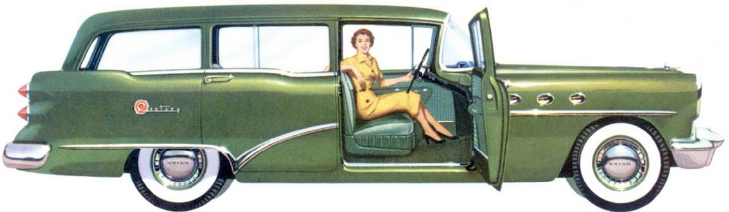
MODEL 69 4-DOOR 6-PASSENGER ESTATE WAGON. 122"-Wheelbase — 200 Horsepower and 8.5 to 1 Compression Ratio with Twin-Turbine Dynaflo, optional at extra cost. 195 Horsepower with Synchro-Mesh Transmission and 8 to 1 Compression Ratio.
