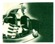
New rubber bushings at the point where the control arms are joined to the frame further aid handling and durability. They reduce noise, dampen road shock and vibration, and eliminate friction and the need for Jubrication.
