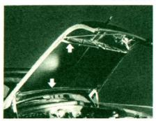
The new one-piece hood has extra sturdiness. A strong bracket is now riveted to the front downward curve of the hood. A new three-piece reinforcement is welded to the rear of the hood.
