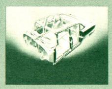
Chevrolet bodies have UNI-TIZED CONSTRUCTION for improved body shell alignment and accurate door fits.
