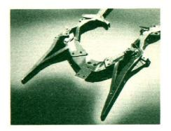
Front and rear cross members are more fully integrated into the frame structure because they are more rigidly attached to the side members.
