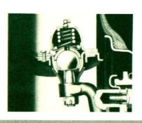
The 1955 Chevrolet uses spherical joints instead of the king pin and control arm outer pivots used on some cars. This allows the wheels not only to turn right and left, but also move up and down with the bumps of the road.
