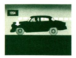
When the brakes are applied on cars without braking dive control, the forward momentum of the car results in a forward transfer of the car's weight and forces the front end of the car downward on the front springs.
