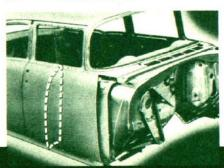
Doors of the new Twin-Guard Body have double-wall construction. Steel-against-steel gives solidness and protection.
