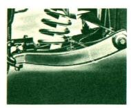
Durability and handling are further improved by the new design of the lower control arm. It has the conventional pan design but it is now upside down so that snow and mud can't collect. This means a freer moving suspension under severe operating conditions.
