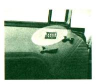
Still another convenience option offered in the 1955 Chevrolet "Two-Ten" and Bel Air Series is Power Control of All Four Windows. There are controls under each window and a master control next to the driver that operates all four windows. Two-speed electric windshield wipers are also available as an option on all models. Another convenience feature available as a separate option is the new power seat control.
