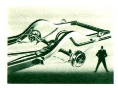
New stability comes from having the rear springs mounted outside the frame. This WIDER spacing of the mountings increases a car's stability just as the spreading of the feet provides a person with increased stability—a charging football linesman for example.
