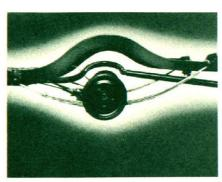
The axle driving forces are first sent to the springs, which flex slightly before passing them on to the frame. This cushions the driving forces before they reach the frame—like the boxer rolling with a punch. This gives new smoothness to Chevrolet's starting, stopping, and cruising.
