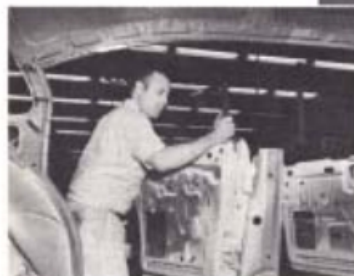
Door window is fitted into place.
