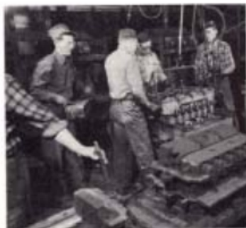
Removing of cylinder block casting from sand mold.
