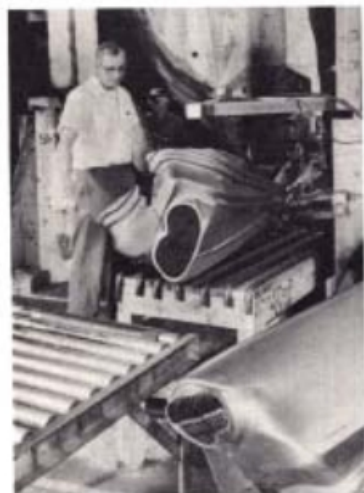
Workman removes front fender from a double-action press.
