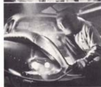
Body joints are spot welded.
