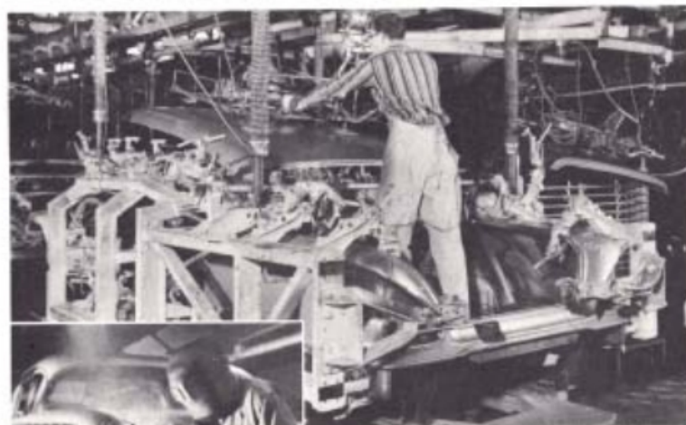
Now the roof meets the body and the car begins to take shape.
