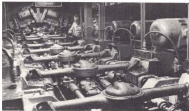
Machines finish outer ends of rear axle housing for wheel bearings and brakes.
