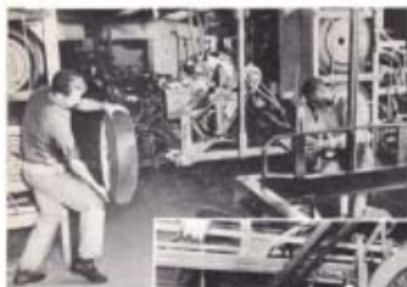
Chassis is now complete and painted wheels are added. This is the first time where the color scheme of the completed car starts to appear.
