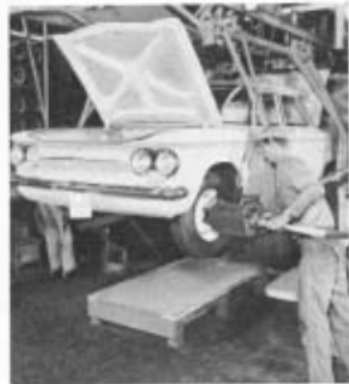
Wheels are added as workmen secure wheel nuts all at one time with compressed air wrench.
