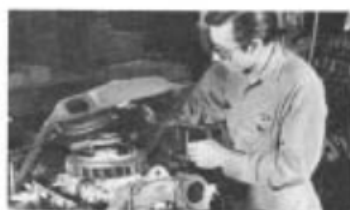
Fan, air shroud and dust shield are added to the Corvaire power train.
