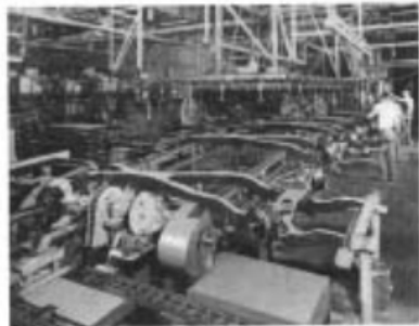
When frame is placed on the line, the assembly operation begins. Workmen attach front end suspension units to frame.
