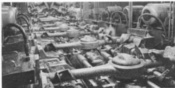
Machines finish outer ends of rear axle housing for wheel bearings and brakes.
