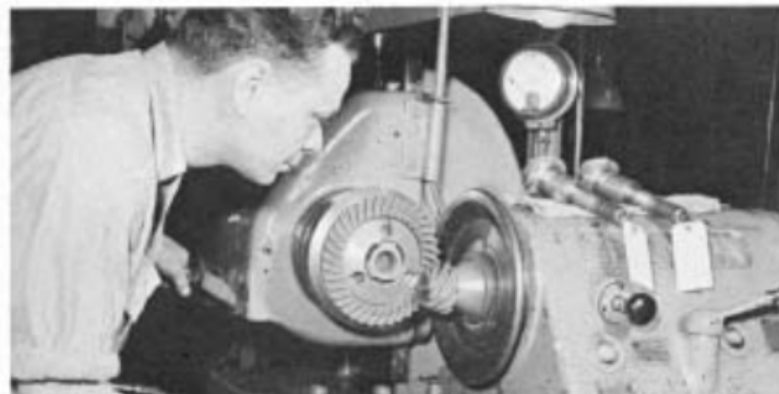
Inspecting ring gear and pinions prior to assembly.
