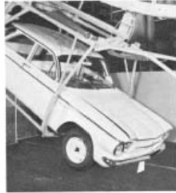
Monorail-cradle dips car down and wheels touch the ground for the first time.
