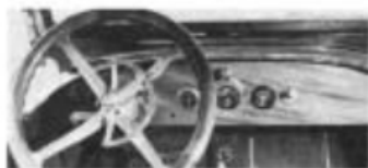
Polished wood steering wheel and instrument panel were standard on the 1918 Chevrolet Touring Car.
