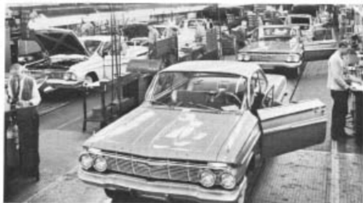
The battery and windshield wipers have been installed. Lights and turn indicators are tested as car assembly nears completion.
