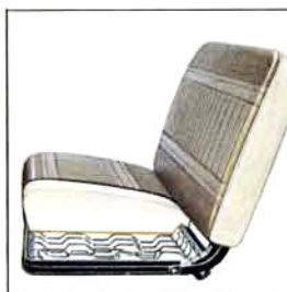
Construction of full-depth foam seat with vinyl upholstery.
