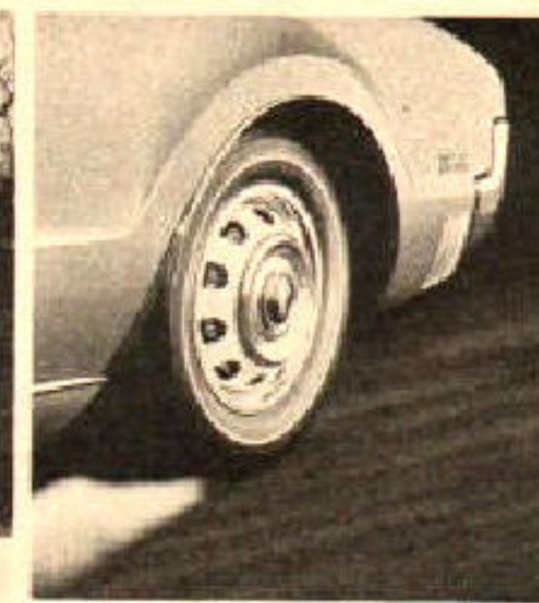
Burly and businesslike! 8.85 x 15 tires, standard, give Toronado a real grip. Wheel cutouts help cool brakes.
