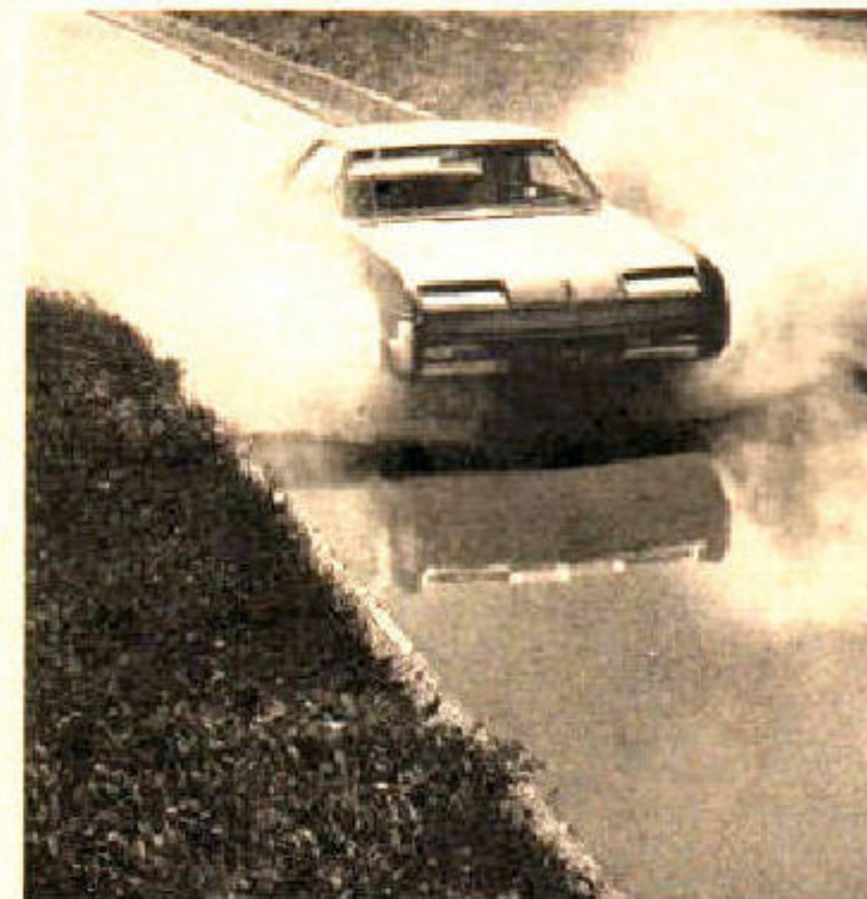
Thorough dunking! Toronado passes water trough test with flying colors! Electrical systems gets the acid test. Salt water checks out corrosion resistance of critical components.
