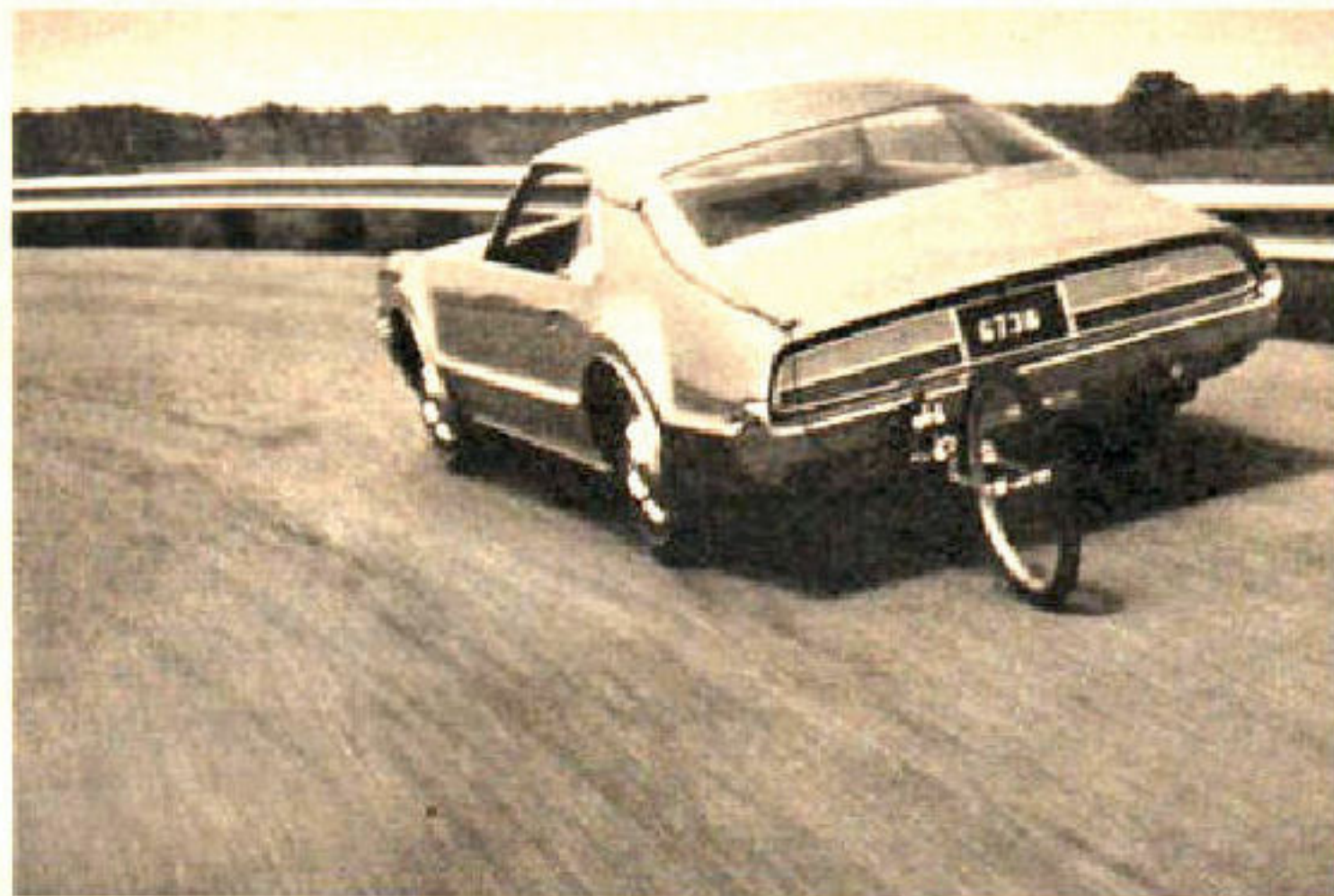
Even a fifth wheel has its function! This one is calibrated to fractions of a mile-per-hour. Records every move the Toronado made in miles and miles of guaging performance around the Proving Ground track. Supplies data for evaluating the test car's response under varying performance conditions.
