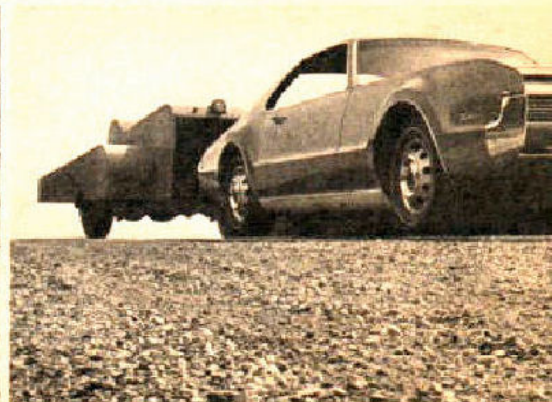
Two-ton tow! Four-thousand-pound dynamometers are towed hour on hour, simulating various grades and driving conditions to produce accurate readings on the road power developed by the 385-hp Toronado Rocket V-8.
