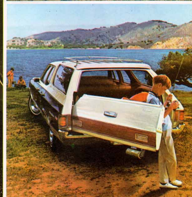
Dual-action tailgate. Above: drops down; below: swings out.
