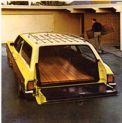
Dual-action tailgate. Above: swings out; below: drops down.
