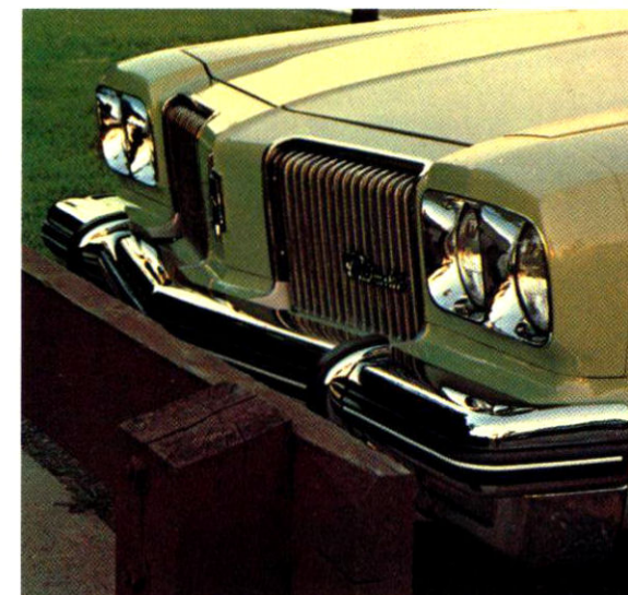
Front and rear bumpers are mounted on hydraulic cylinders which telescope in to absorb minor impacts, then return bumper to original positions.
