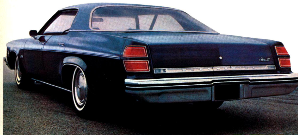
With taillamps stacked vertically in the fenders, Delta 88's trunk opening comes clear down to bumper height across its full width—requires less lifting than some other cars to clear the sill.
