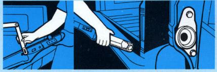
**CHEVY** quick-release tailgate is easily removed by one person without tools—especially helpful to campers. Just release retaining straps, lift up on right side and pull out at left side. To reinstall, simply reverse procedure.
