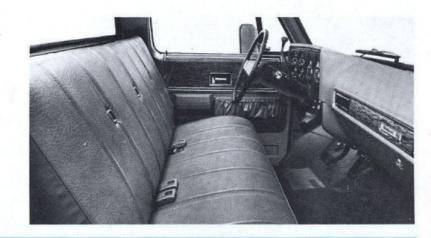
CHEVY dash has three instrument clusters. Each may be removed individually from the front for easy replacement or repair.
