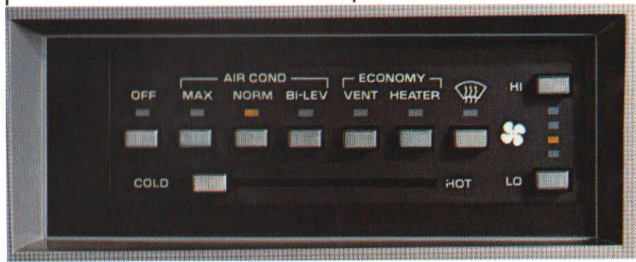
Air conditioning with new push-button controls.
