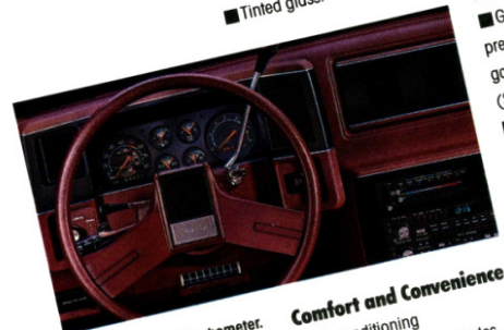
Gage package with tachometer. (Std. on SS)
