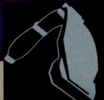
Grand Prix's carbon-strand and fiberglass composite rear leaf spring is a single-leaf arc that's lighter and stronger than steel. It uses less space and adds more roll stiffness than conventional coils.
