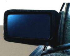
Hot cars deserve appropriate side mirrors, so those of SSE are heated to aid defrosting and tinted blue to cut glare day and night.
