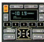
UM7: Delco ETR® AM/FM stereo radio with seek up/down, and digital clock.
