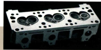
The 2.8L V6 cylinder head is cast in aluminum for light weight. High-efficiency canted valve configuration gives a swirl to the incoming air-fuel mix for a fast, even burn.
