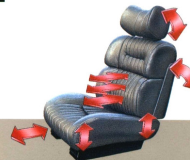
Attitude adjustment can be achieved 12 different ways with SSE's power articulating seat. Inflatable bladders inside respond to console switches and tailor the seating comfort to you.
