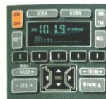
U1C: Delco ETR® AM stereo/FM stereo with seek/scan, compact disc, and digital clock.
