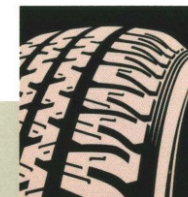
Standard GSE wheel "attire" is the P185/60R14 82H Euro-design blackwall. It's "H" rated for high performance.
