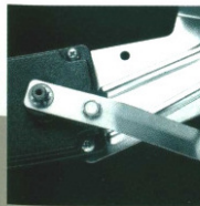
STE drivers are always on the level thanks to this special switch, mounted to the car's rear subframe. It can detect excessive rear down-loading, activate an air-pressurized system, and restore level ride attitude.
