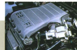
The 2.8L V6 features multi-port fuel injection, crank-triggered, triple-coil ignition and a wagon-hauling team of 125 horsepower.
