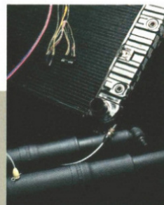
Tow a trailer? Delco Superlift air shocks, a seven-wire trailer harness and the extra-cooling radiator are part of Safari's available trailering equipment.
