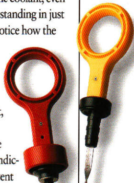
Here’s one more common-sense innovation: a spin-off fluid filter on the automatic transmission. It not only makes the filter easier to change, but keeps you from having to remove the bottom pan—a procedure that can cause leaks.
