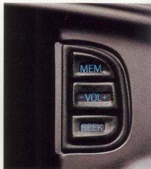
The driver has a separate stereo control module (volume, seek, memory) on the instrument cluster.
