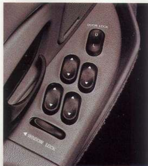
Optional power windows/locks now have lighted controls. Driver's window has new "express-down" feature.
