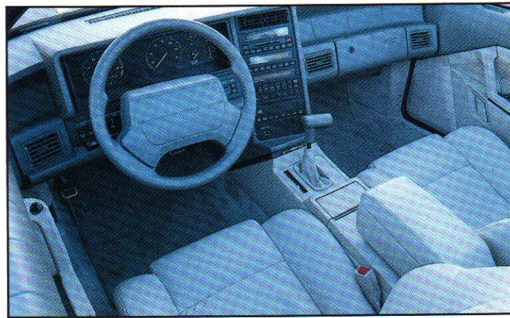
New seats (left) offer power lumbar support. Other comfort and convenience changes include a cup holder in console, easier access to interior cargo space. Dash has been changed so tach and speedometer readings keep pace with capacity of new engine
