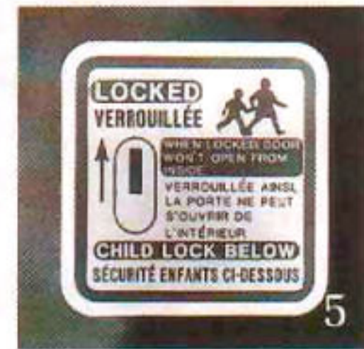
5. Activating the child-proof door locks keeps children in back from opening the rear doors from inside the car, while allowing doors to still be opened from outside.
