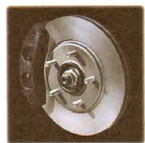
All Cutlass Supremes feature standard anti-lock brakes which prevent wheel-lockup, thereby helping the driver maintain steering control under maximum braking conditions, even on wet or other slippery surfaces.
