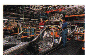
If you could peel back the glossy skin of your Saturn, you'd see this reinforced steel passenger cage—the formidable Saturn spaceframe. With crumple zones fore and aft to help absorb front and rear impacts, it also houses energy-absorbing bolsters in the dash to cushion knees; ramps in the rear seats to help keep small people from sliding forward and under their belts; and dual airbags.
