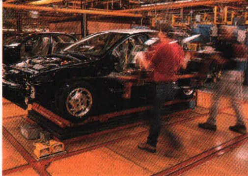
At Saturn, instead of struggling to attach parts to a car that's passing by on a conveyor belt, our factory technicians can move with the car, by riding on "skillets"—comfortable wooden platforms like the orange ones you see in the photo above. What's more, these skillets come with pneumatic lifts, which means the technicians can raise and lower the entire car to the height most ergonomically comfortable for them. The way we see it, the happier our team members are, the happier you'll be in the end.
