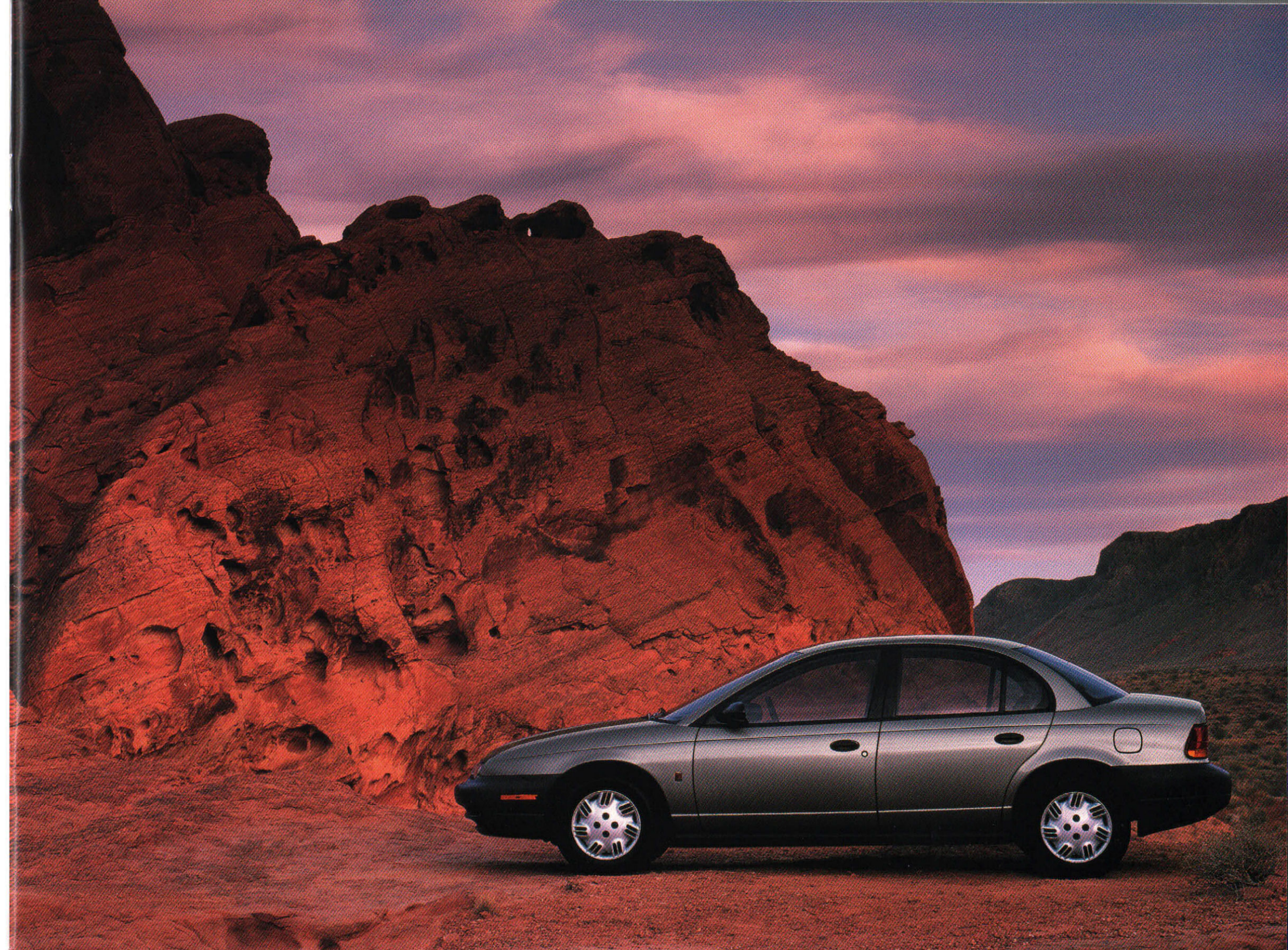
Dent-resistant polymer body-side panels are among the design team's more intriguing innovations. The panels are painted with a primer coat that flexes on impact, a waterborne acrylic color basecoat that looks wet and lustrous, and a clearcoat tough enough to fend off tree sap, ultraviolet light, and even the most wayward pigeon. Recyclable and resilient, they won't rust, oxidize, or fall prey to the usual nicks, dents, or dings inflicted by such everyday hazards as shopping carts, car doors, or even young Monica, the budding neighborhood T-ball champion.
