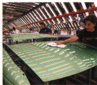
Dent-resistant polymer body-side panels are among the design team's more intriguing innovations. The panels are painted with a primer coat that flexes on impact, a waterborne acrylic color basecoat that looks wet and lustrous, and a clearcoat tough enough to fend off tree sap, ultraviolet light, and even the most wayward pigeon. Recyclable and resilient, they won't rust, oxidize, or fall prey to the usual nicks, dents, or dings inflicted by such everyday hazards as shopping carts, car doors, or even young Monica, the budding neighborhood T-ball champion.
