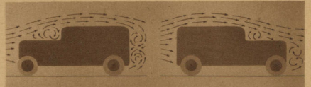
DIAGRAM ILLUSTRATING that the conventional motor car would travel faster if the position of the body were reversed, because of lessened wind resistance.
