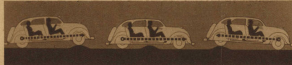
THIS DIAGRAM illustrates what happens when an Airflow Chrysler car goes over a bump and why the new ride made possible by the Airflow design is superior to all others.
