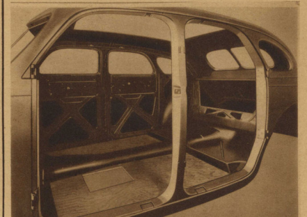
BODY, FRAME AND SILL are welded into one unit in the girder bridge type construction used in the Chrysler Airflow cars. Body panels and cross members are electrically welded, trussed and braced with steel at all points of stress.
