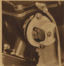
MANIFOLD HEAT CONTROL thermostat, one of the features contributing to the efficiency of the 1934 Chrysler power plant.
