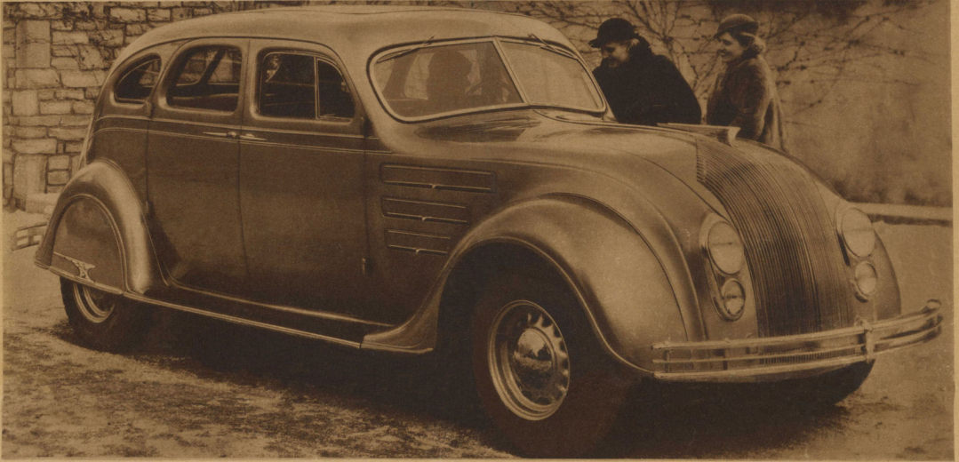
CHRYSLER'S CROWNING ACHIEVEMENT—the tenth anniversary Airflow Chrysler Eight 4-Door Sedan, called by Walter P. Chrysler “the first real motor car since the invention of the automobile.” This car has a wheelbase of 123 inches and 122 horsepower.
