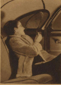
REAR SEAT PASSENGERS in the Airflow Chrysler Eights control their own ventilation by means of adjustable quarter windows. This is a feature of the new Chrysler Draft-Free ventilation system.
