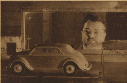
ALEXANDER WOOLLCOTT, playwright, author and actor, learns what the Airflow Chrysler design means in lessened wind resistance by watching a model in the air tunnel.
