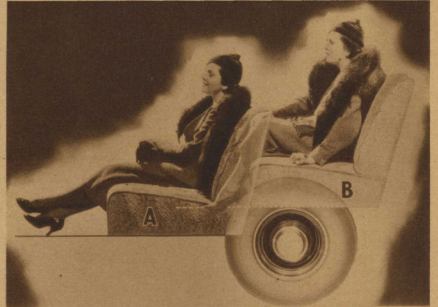
ONE OF THE ENTIRELY NEW PRINCIPLES found in the new Airflow Chrysler Eights. Figure "A" shows where rear seat is placed in these new Chryslers; figure "B" where it is placed in the conventional car. Putting this seat 20 inches in front of the rear axle makes an indescribable difference in riding comfort.
