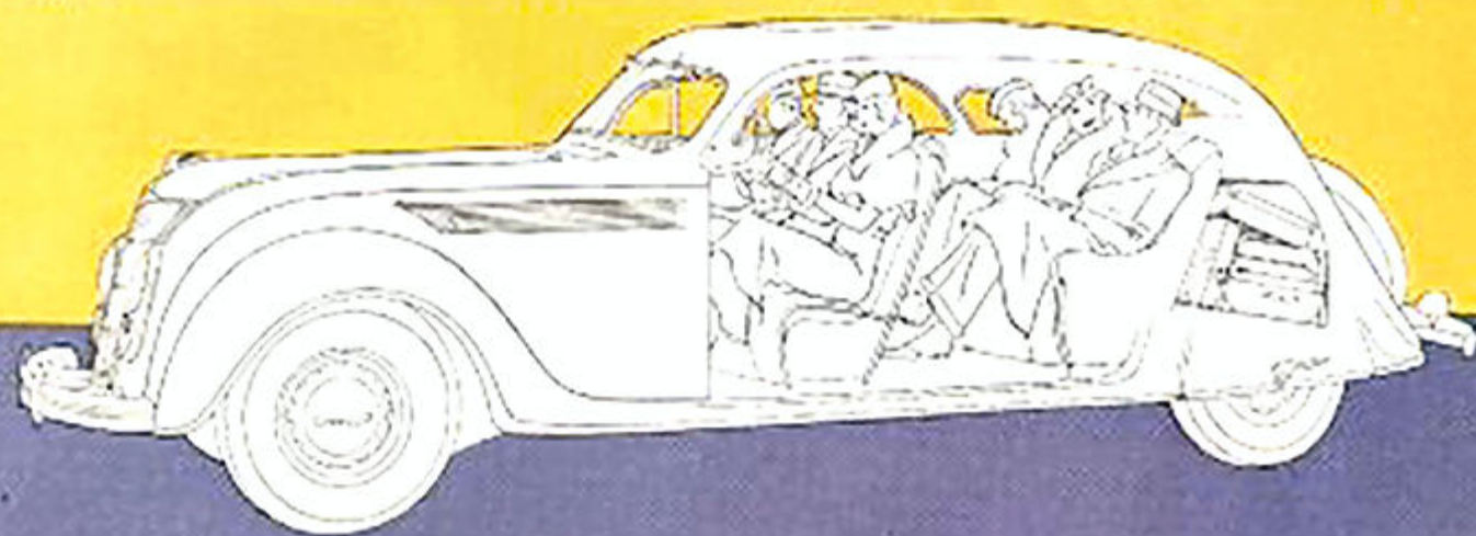
Passengers are cradled between the wheels at the point of minimum perpendicular action.
