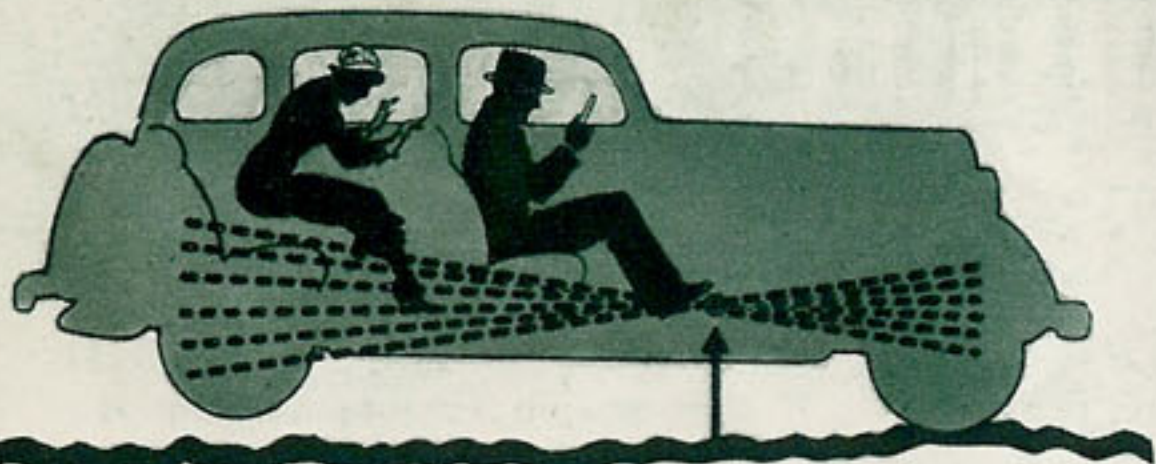
The old way. Stiff front springs and 60 per cent of weight on rear springs caused front end bounce.
