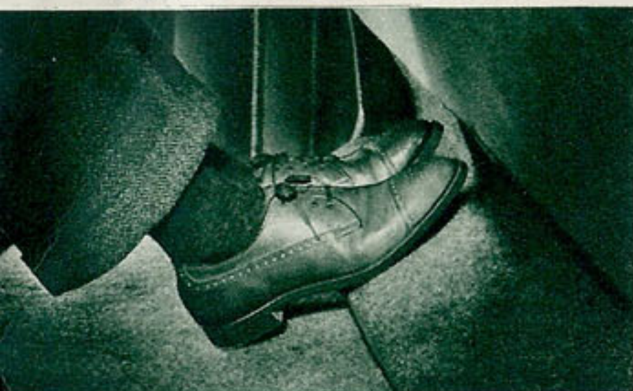
FOOT CLEARANCE! For tall people extra provision is made in this foot rest recessed into the rear of front seat.
