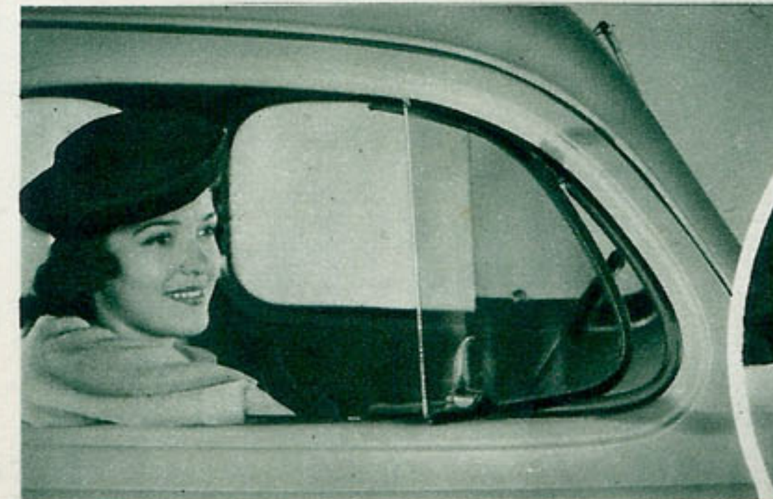
IF YOU WANT A BREEZE! Swinging the ventilating wings out scoops in the air. No crank to turn to adjust the ventilating wings. Simply push them into position and there they stay. Rear section of window lowers completely. Lock firmly secures latch when wing is closed.
