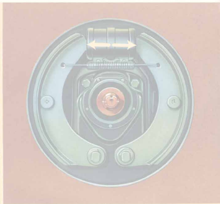
Straight-line trips are favored by equal pressure hydraulic brakes.
