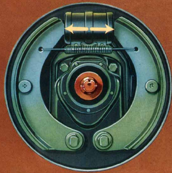
Straight-line stops are insured by equal pressure hydraulic brakes.
