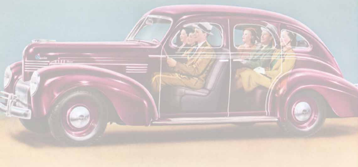
In the new Chrysler, the rear seat is placed forward of the axle, so that passengers ride in cradled comfort.
