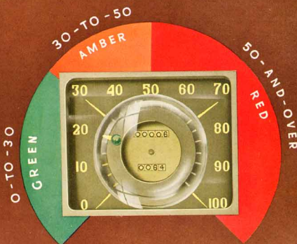
The new safety speedometer signals car speed day or night.
