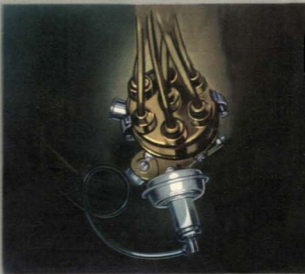
Vacuum control automatically advances and retards the spark to give maximum efficiency and economy under all driving conditions.
