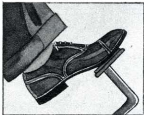
When a driver applies the brakes, he can measure and regulate stopping force only by means of "pedal feel."
