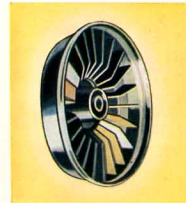
The front fanlike wheel of a Chrysler Fluid Drive unit is a small replica of the turbine wheel and transmits power in exactly the same way as in a power plant.
