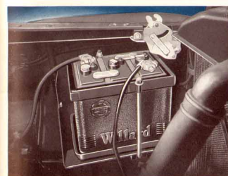
Battery. Located forward under hood—for easy accessibility without disturbing passengers. Air vent caps prevent overfilling.
