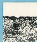
A profile of a piece of metal prepared by grinding, when viewed under the microscope, shows surface indentations.
