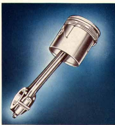
Standardized Aluminum Alloy Pistons. Superfinished and then coated with pure tin, to prevent scuffing or scoring.
