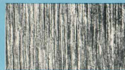
Metal prepared on a grinding wheel, when photographed under a microscope in a cross light, is rough, grainy and scratched with ridges. These surface defects mean close fits are impossible—mean increased friction because the ridges rupture the protecting oil film.
