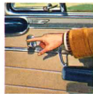
Electric Window Lifts, with separate motor on each window, available at extra cost.
