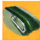
Assist handles, rigidly mounted on front seat back, are a safety and convenience feature.
