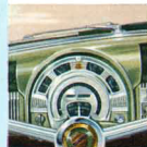
The Safety-Eye Instrument Cluster, with all gauges grouped to be read at a glance.
