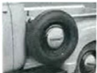
Side Mounted Tire Carrier —Convenient location for spare wheel and tire. Available for pickup models 3104-3604 and 3804.
