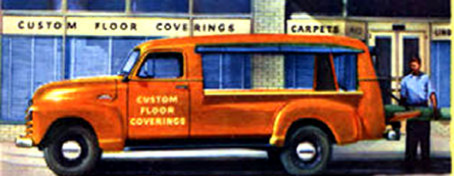
MODEL 3807 CANOPY EXPRESS 137" W.B., MAX. G.V.W. 7000 LB. Over-all dimensions are similar to those of 3805, Panel
