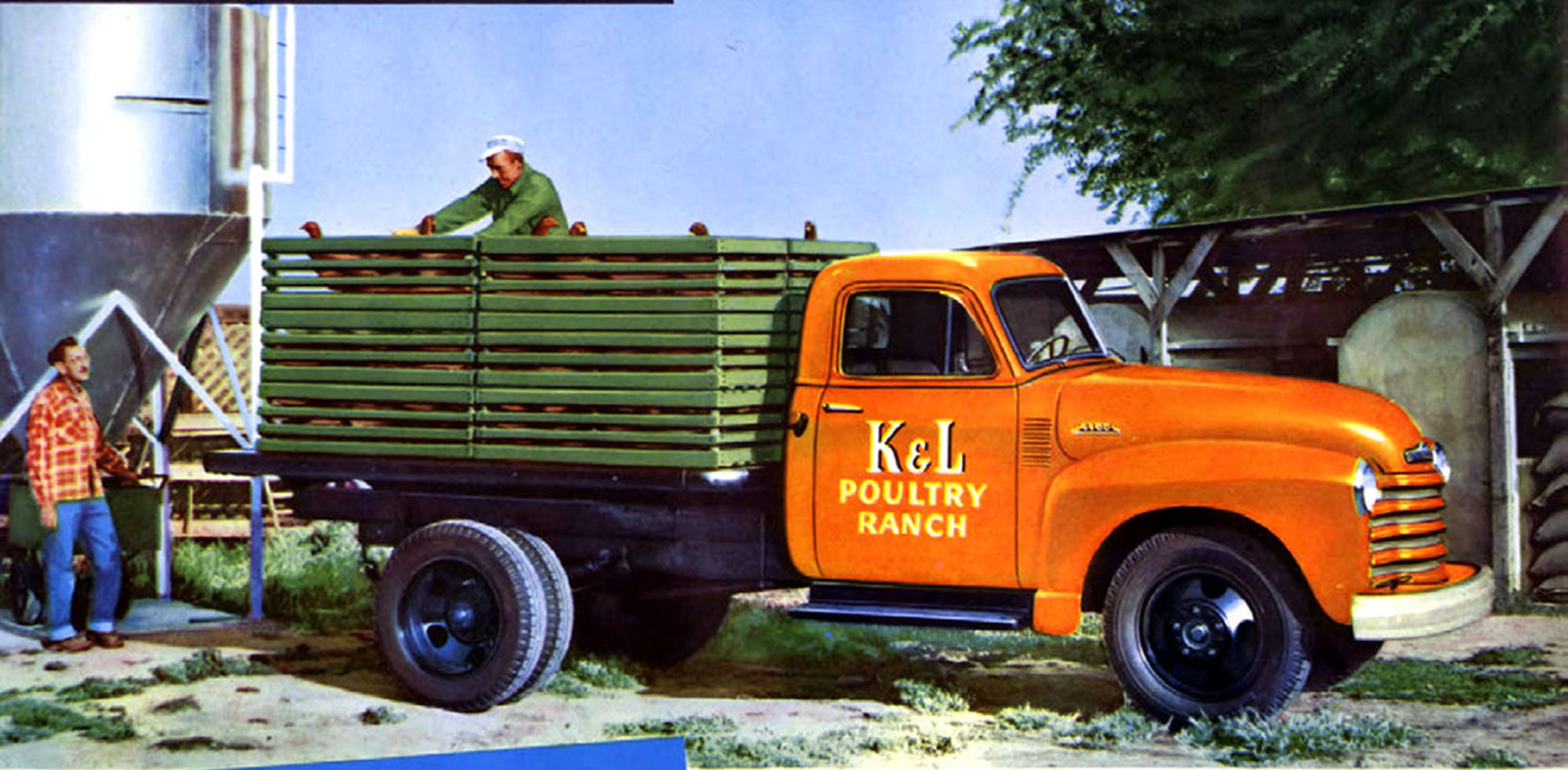
MODEL 4108 PLATFORM 137" WHEELBASE, MAXIMUM G.V.W. 14,000 LB. Also available: 4109 Stake Truck and in 6100 Series
