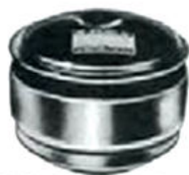
Oil-Bath Air Cleaner —A heavy-duty unit for trucks that operate in dusty regions.
