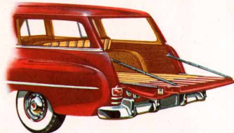
Tailgate opens flush with floor for easy loading or unloading. Width of storage space 47 inches; height 35 inches. Length rear seat to tail gate 75 inches.
