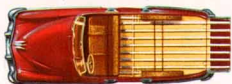
Either half of divided rear seat, or both, can be folded forward to form flat storage compartment 116 inches long.
