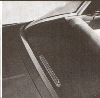
REAR WINDOW DEFROSTER clears fog, frost, dew. Two-speed motor for efficient operation.
