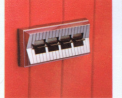
Power Windows can all be operated from driver's seat. Individual control at each window.
