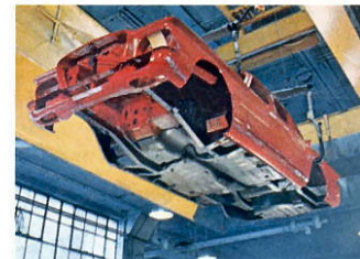
Valiant's rugged one-piece Unibody is dipped and sprayed 13 times to help prevent costly corrosion.
