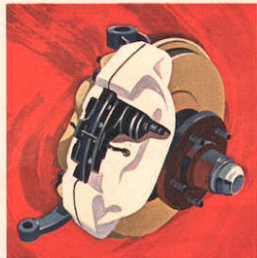
Front-Wheel Caliper-Type Disc Brakes for tough service.
