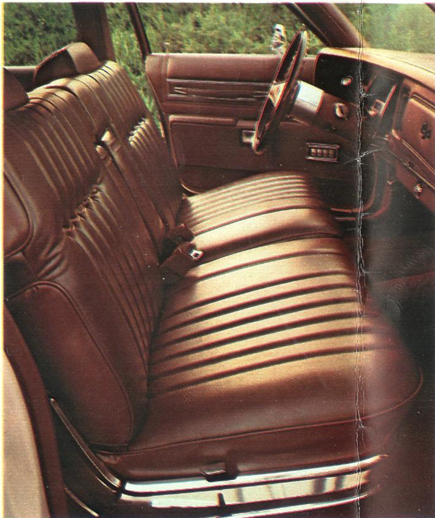
Standard vinyl 50/50 bench seat, with folding center armrests, and reclining passenger-side seat.
