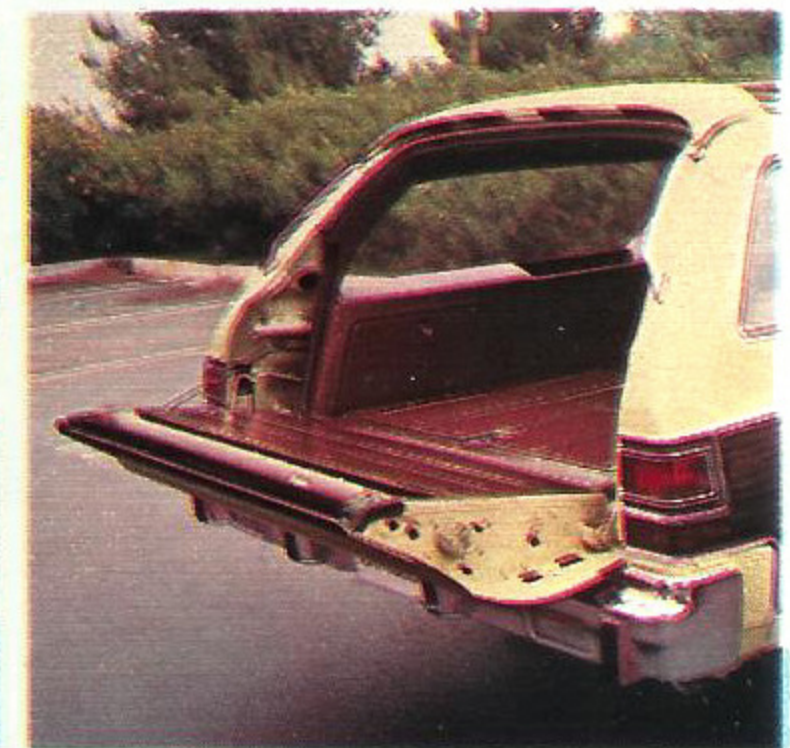
Three-way doorgate is standard. When dropped down, doorgate is almost level with cargo floor for easy access and loading.
