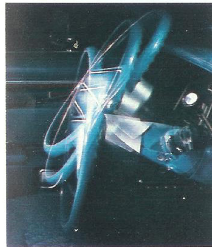
Tilt & Tel Steering Wheel, shown here in three positions. (Gran Fury / Town & Country only.)
