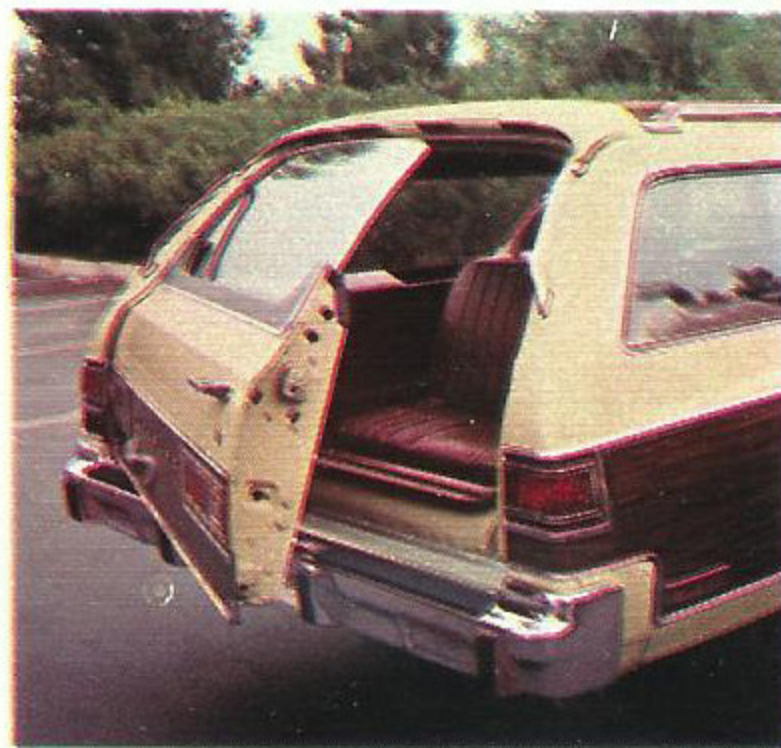
Three-way doorgate is standard. When dropped down, doorgate is almost level with cargo floor for easy access and loading.
