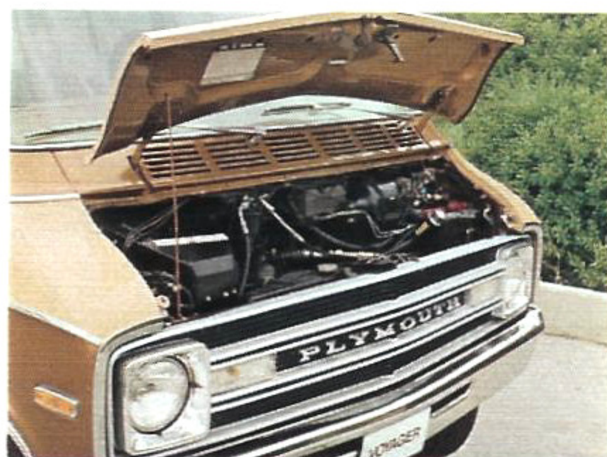
Large engine hood makes service access simple and easy for maintenance and repair work.
