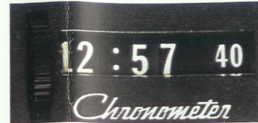
Electronic Digital Clock is accurate to within one minute per month. (Town & Country and Gran Fury only.)
