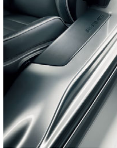
Door sill panels in body colour with nappa leather insert and embossed AMG lettering
