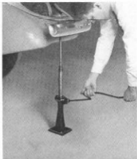
New Type Jack, Fitting Conveniently Under Bumper Bracket
