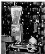
Weighing Connecting Rod
