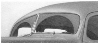
New Vacuum-operated Windshield Wipers (Clear Semi-circle Shows Wiper's Range)
