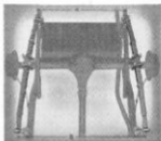
Splayed Springs (Note Greater Width at B than at A)
