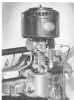
Down-draft Carburetor, Radial Manifold, Automatic Choke, Vapor-lock Relief Valve, Air Cleaner and Silencer, and Backfire Arrester
