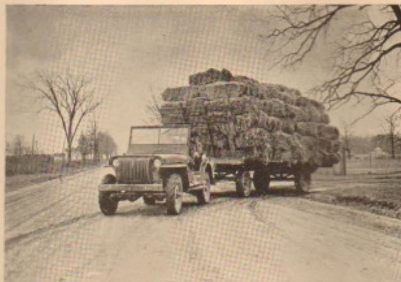
Especially effective in hauling trailer loads over the highway, the Jeep can pull 5500 pounds at a rapid rate with sufficient power to meet steep grades and bad road conditions.
