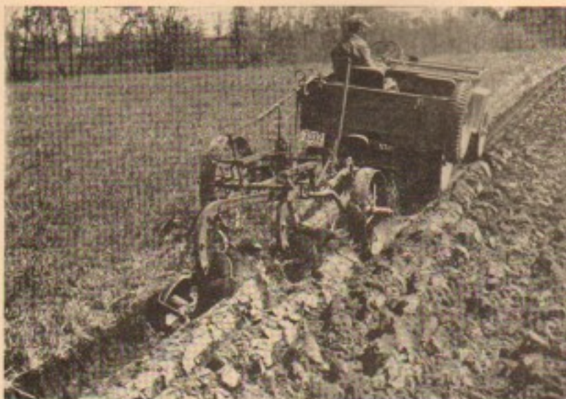
Adapted for continuous service in the field, the Universal Jeep is shown operating a two-bottom, 12-inch plow. It is equally effective with the single bottom, 18-inch plow.
