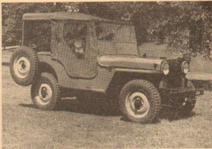
Detachable front and rear tops afford the Jeep driver and passengers all-weather protection. A heater, 3-inch seat cushions, telescopic type shock absorbers and more flexible springs are other comfort features available in the peacetime model.
