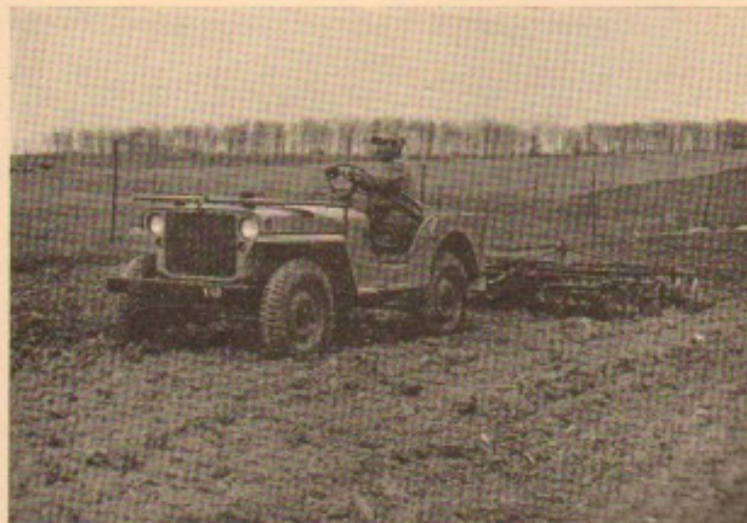
The Jeep is equally at home pulling a tandem disc harrow as it was drawing a 75 mm. gun. Unbooked from a harrow or other tillage tools, the vehicle carries on as a light truck, mobile power unit or passenger conveyance.
