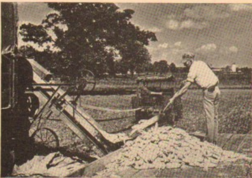
A special power take-off, which can be used with a spline shaft for direct power or with a belt pulley, makes it possible for the Jeep to delegate up to 30 HP to anything from a buzz saw to a corn sheller, such as it is shown operating.
