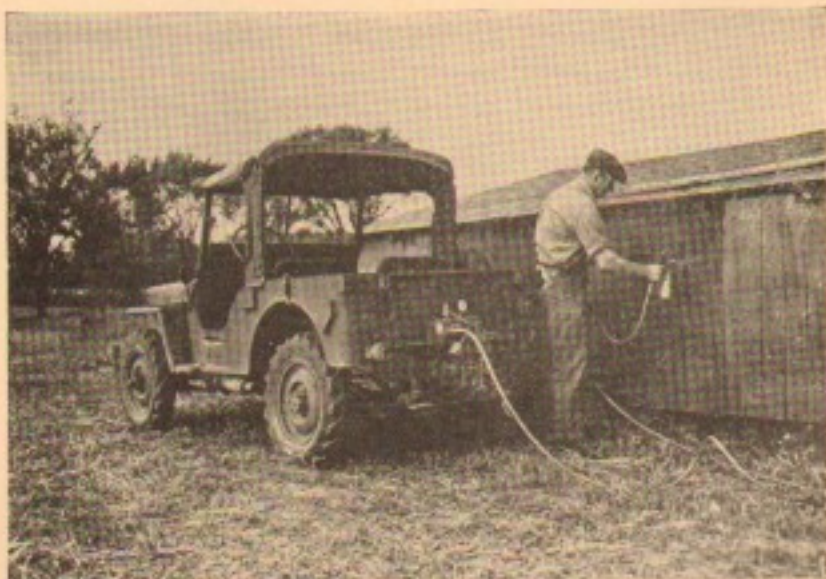
The Jeep supplies ready and mobile power for use in spray painting barns, fences and other surfaces requiring care and attention on the farm.
