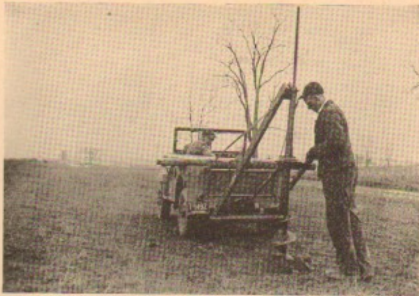
The Jeep supplies relief in the elimination of back-breaking jobs on the farm as typified by this post hole auger which operates from the power take-off shaft.
