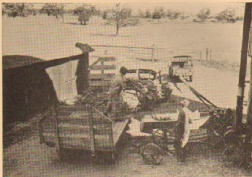
The Universal Jeep provides power to operate silo filler with cutter. With corn bundles being tossed into the cutter from the trailer behind the second Jeep the 40-foot silo was filled to its 125-ton capacity in less than 16 hours.
