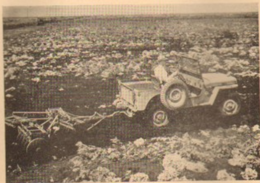
Pulling a disc harrow through heavy muck soil of Florida was part of the extensive tests devised for the Universal Jeep at agricultural experimental stations throughout the country.
