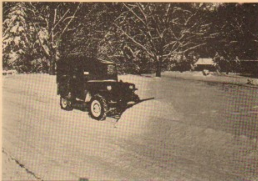
Outfitted with a snowplow attachment, the Universal Jeep fulfills the promise of its capacity for around-the-year work by keeping a country road open.
