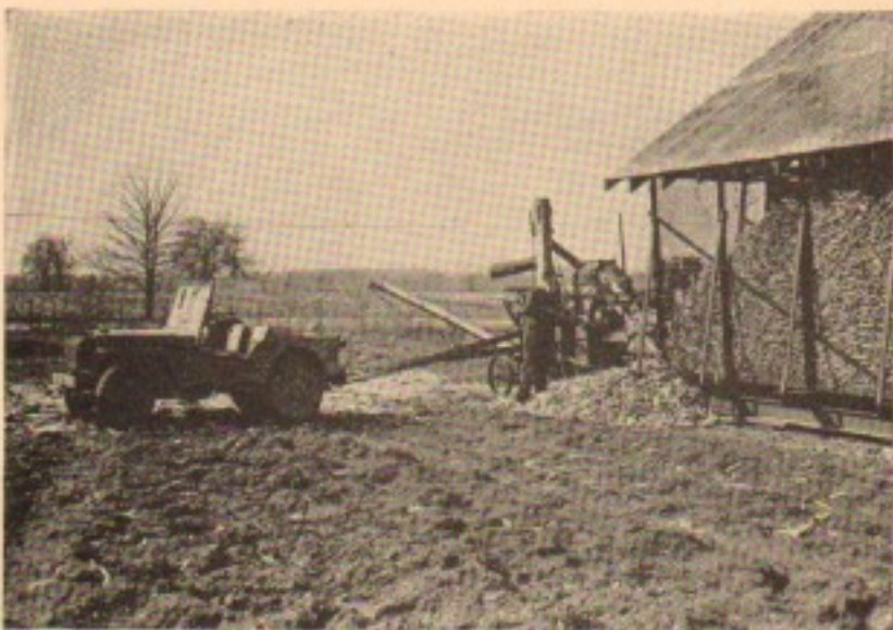
The Universal Jeep, designed by Willys-Overland Motors, furnishes power for corn shelling. A belt-driven governor is available and can be installed wherever constant engine speed, regardless of load, is needed.
