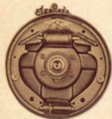
Above: Servo-action design increases power.
