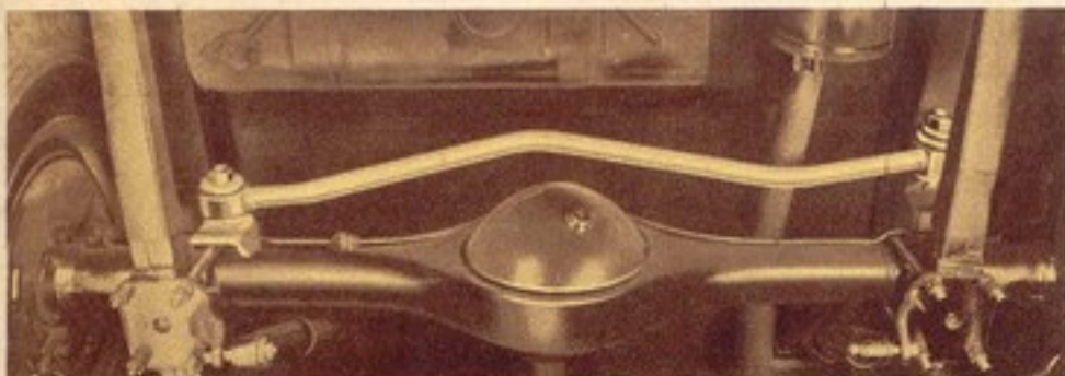
Rear stabilizer bar is rubber-cushion mounted on body-and-frame foundation member at top and on axle housing at bottom.
