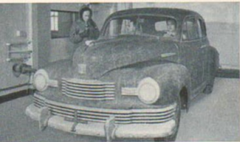
Completely equipped laboratories duplicate the most difficult operating conditions. Here engineers are testing cold-weather operation in temperatures 40° below zero.
