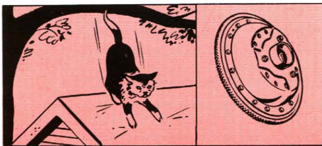
Cat's-paw action in Hudson clutches is provided by cork friction surfaces
