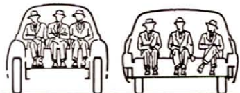
Body on top of frame. High roof and high center of gravity.
