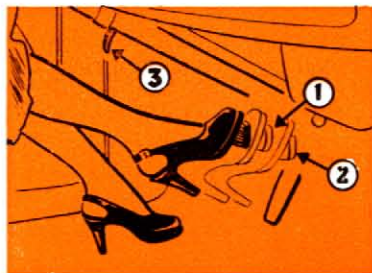
Hudson's Triple-Safe Brakes: 1) pedal operating hydraulic brakes, 2) same pedal operating mechanical reserve brakes, 3) finger-tip-release parking brake.
