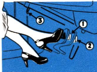
Brake pedal travel (1) for hydraulic brakes, (2) for mechanical reserve brakes. (3) Parking brake handle.
