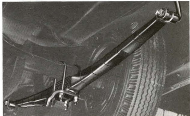
Hudson's long, leaf-type, metal-covered rear springs, mounted in splayed position.
