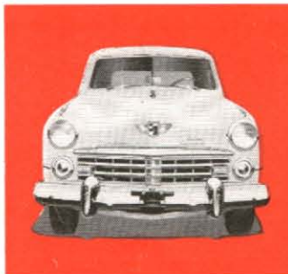
Studebaker Land Cruiser with body-over-frame design is higher, narrower, and has less interior room.
