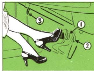
(1) Pedal travel for hydraulic brake operation. (2) Pedal travel for reserve brake operation. (3) Finger-tip-release parking brake.
