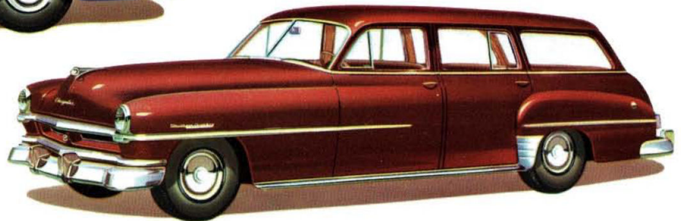
THE TOWN & COUNTRY WAGON . . . the smartest and most serviceable station wagon on the road. Divided seat in rear compartment folds forward giving large luggage space. Tailgate lowers for rear loading.
